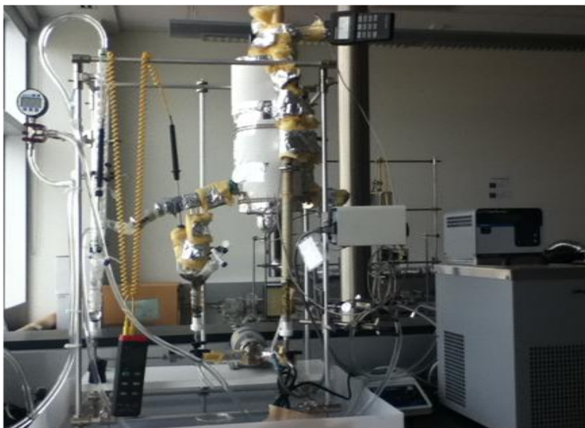
Figure 3.1 Experimental setup of the Swietoslowski Ebulliometer
