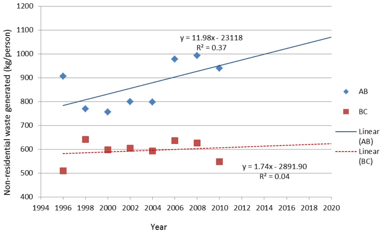
Figure 4.7: Linear model of non-residential waste generated per capita in Alberta and British Columbia
