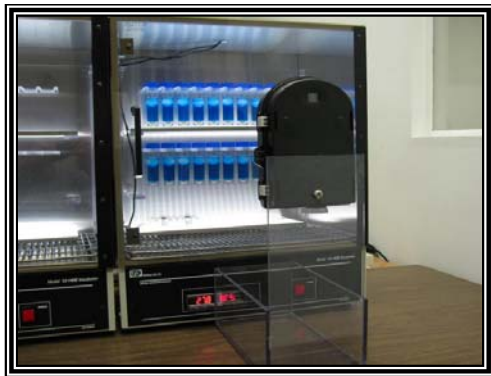
Figure 1. VBR II including an advanced temperature controlled unit.
