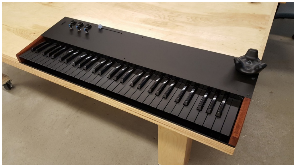
Figure 8. The Mixed Reality MIDI Keyboard.
